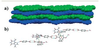
Fig. 7 a) Molecular layers of TBR-2(4HBA)- $H_2O$ , which are held by  $\pi \cdots \pi$ interactions (blue and green colors indicate the layers composed of I II hydrate systems, respectively); b) representation of  $\pi(TBR)\cdots\pi(K4HB)$  interactions in the  $TBR\cdot2(4HBA)\cdot H_2O$  cocrystal hydrate.
