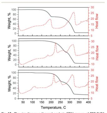
Fig. 12 The simultaneous thermal analysis (STA) curves of TBR-2HBA (top), TBR-3HBA (center) and TBR-2(4HBA)- $\rm H_2O$  (bottom). TG and DSC curves are represented by black and red colors, respectively.
