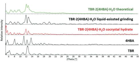
Fig. 11 Comparison of powder X-ray diffraction patterns for theobromine, 4-hydroxybenzoic acid and the TBR-2(4HBA)-H<sub>2</sub>O cocrystal hydrate.
