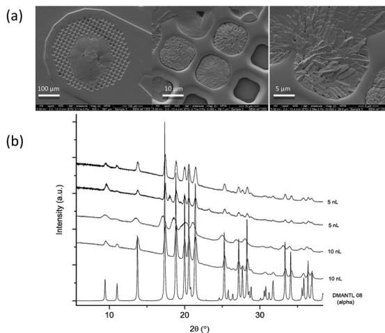
**Fig. 3** (a) SEM images of crystals formed in printed droplets on an XRD mesh (10 nL) and (b) XRD patterns for crystals formed in printed 5 and 10 nL droplets showing characteristic peaks for the  $\alpha$  polymorph (calculated reference PXRD patterns for mannitol polymorphs are given in Fig. S2†).
