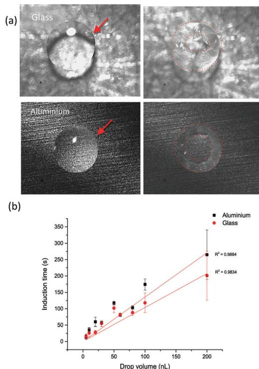
**Fig. 5** (a) Images of 100 nL droplets on glass and aluminium foil substrates with the red arrow indicating the point of start of crystallisation and red dotted-line circles indicating coffee-ring formation during droplet drying, and (b) crystallisation induction time as a function of drop volume in droplets printed on both substrates.
