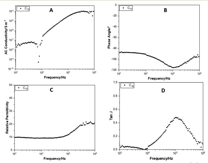
Fig. 12 Change in (A) AC conductance, (B) phase angle, (C) relative permittivity and (D)  $\tan \delta$ , over a frequency sweep range of  $10^3$ – $10^6$  Hz, for TBAFC<sub>10</sub>.
