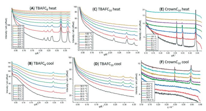
Fig. 10 Heat-cool 1D SAXS profiles. (A and B) TBAFC<sub>8</sub>; (C and D): TBAFC<sub>10</sub>; (E and F) CrownC<sub>10</sub>. Profiles are offset on the vertical axis for clarity.
