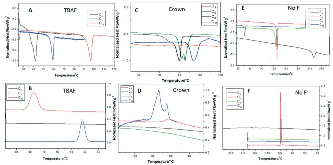
Fig. 2 DSC thermograms of (A) heating of TBAF compounds; (B) cooling of TBAF compounds; (C) heating of crown compounds; and (D) cooling of crown compounds. POSS without F<sup>-</sup> ion encapsulation (E) heating cycle and (F) cooling cycle.
