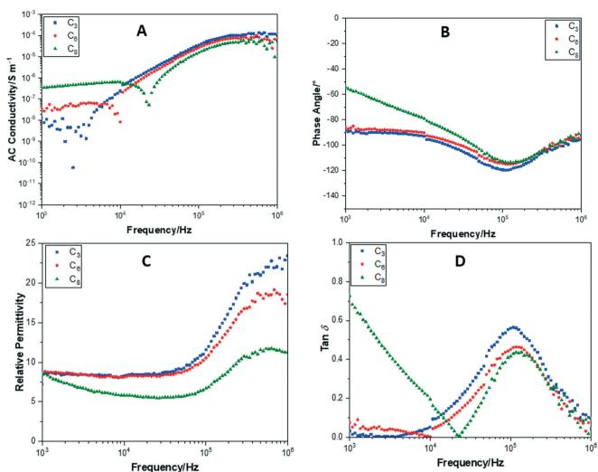
Fig. 13 Change in (A) AC conductance, (B) phase angle, (C) relative permittivity and (D)  $\tan \delta$ , over a frequency sweep range of 103-106 Hz, for CrownC<sub>3</sub>, CrownC<sub>6</sub> and CrownC<sub>8</sub> compounds.
