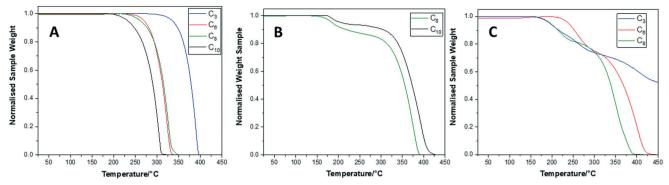
Fig. 4 TGA curves of (A) POSS compounds without F<sup>-</sup> ion encapsulation, (B) TBAF compounds and (C) crown compounds
