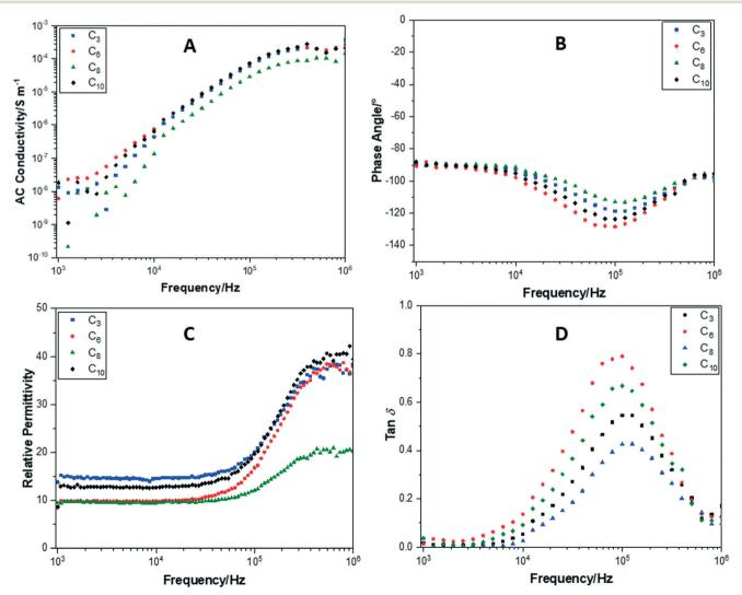
Fig. 11 Change in (A) AC conductance, (B) phase angle, (C) relative permittivity and (D)  $\tan \delta$ , over a frequency sweep range of  $10^3$ – $10^6$  Hz, for POSS compounds with fluorinated alkyl chain arms (without F<sup>-</sup> ion encapsulation).
