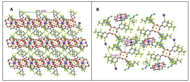
Fig. 8 2D polymeric network packing in (A)  $CrownC_3$  and (B)  $CrownC_6$  compounds from single crystal X-ray packing analysis.<sup>11</sup>
