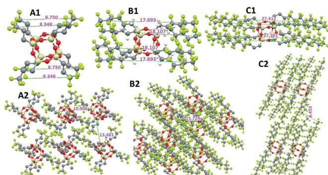
Fig. 9 Estimated molecular dimensions and packing scenarios of POSS with fluorinated alkyl chain arms: (A1 and A2) C3 arm length, (B1 and B2) C<sub>6</sub> arm length and (C1 and C2) C<sub>8</sub> arm length.
