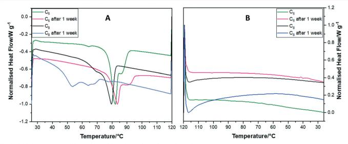
DSC thermograms of (A) heating and (B) cooling of CrownC<sub>6</sub> and CrownC<sub>8</sub> samples over a week.
