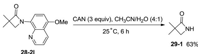
Scheme 29 Oxidative cleavage of the 5-methoxyquinolyl group.
