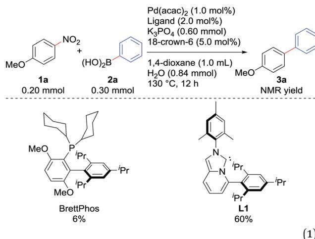
To make this system more efficient, we made an attempt to use (**L1**)Pd complexes as catalyst precursors (Table 1). (**L1**)Pd(acac)Cl was prepared and examined first, but the yield was similar to the case where Pd(acac)<sub>2</sub> and **L1**·HCl were independently used. Another complex (**L1**)Pd(allyl)Cl proved to be effective to afford **3a** in 76%.
