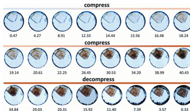
**Fig. 2** Optical transmitted-light micrographs of a MTO single crystal view through a diamond anvil cell in the course of compression and decompression in a silicone oil pressure medium. The diameter of the sample chamber is around 110  $\mu\text{m}$ .
