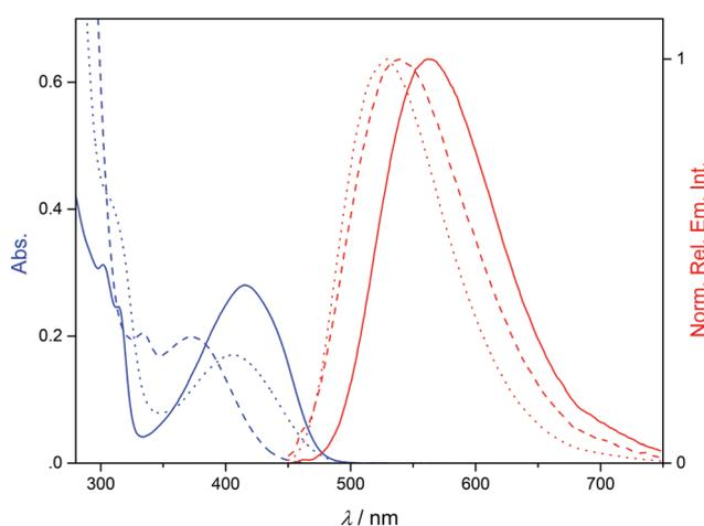
**Fig. 1** Absorption (blue, *c* = 40  $\mu$ M) and emission spectra (red, Abs. = 0.10 at  $\lambda_{\text{ex}} = 405$  nm) of **2a** (solid line), **2b** (dashed line) and **2c** (dotted line) in MeCN.
