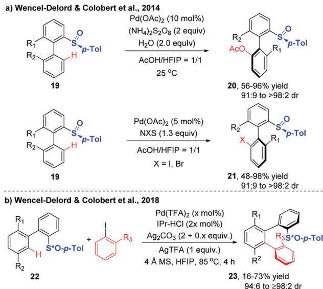
Scheme 9 Chiral sulfoxide-directed diastereoselective C–H acetoxylation, halogenation and arylation (Wencel-Delord and Colobert et al.).<sup>19,20</sup>
