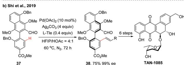
Scheme 12 Pd-Catalyzed atroposelective C–H olefination of biaryl aldehydes using Tle as a transient chiral auxiliary (Shi et al., 2017, 2019).<sup>25,26</sup>
