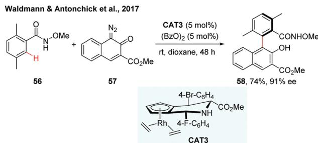
Scheme 17 Synthesis of axially chiral biaryls by Rh-catalyzed enantioselective C–H arylation (Waldmann and Antonchick *et al.*, 2017).<sup>34</sup>
