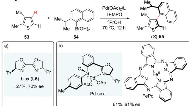
Scheme 16 Enantioselective C–H coupling of thiophene with arylboronic acid (Yamaguchi and Itami *et al.*).<sup>32,33</sup>
