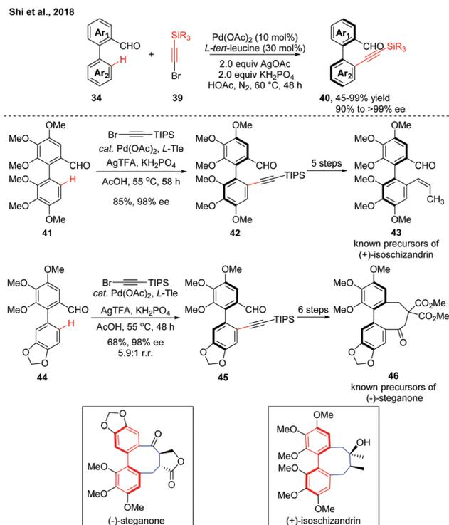
Scheme 13 Pd-Catalyzed atroposelective C–H alkylation and its synthetic applications (Shi et al., 2018).<sup>26</sup>
