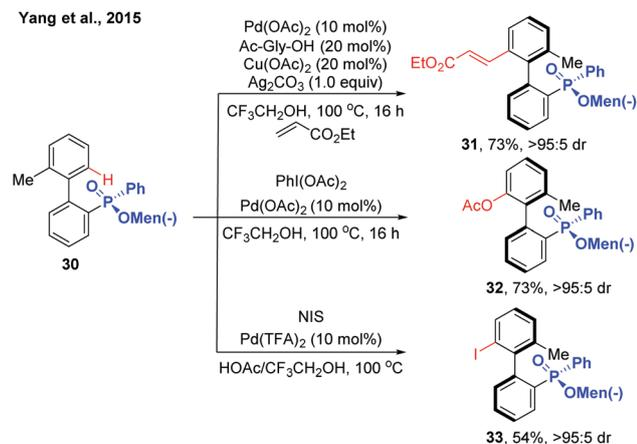
Scheme 11 Pd(II)-Catalysed menthylphenylphate-directed C–H activation/dynamic kinetic resolution for the synthesis of chiral biaryl phosphates (Yang et al., 2015).<sup>21</sup>
