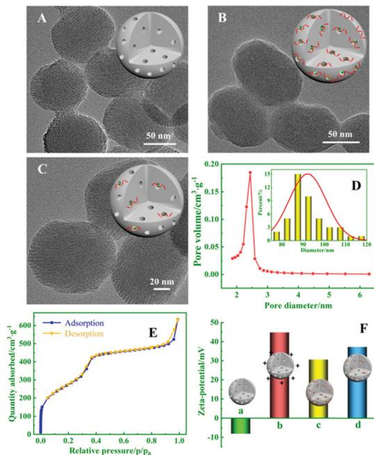
Fig. 3 TEM images of MSNs (A), CsDNA-capped PMSNs (B), and CsDNA-capped PMSNs in the presence of miRNA-21 (C); (D) pore size distribution (inset: size distribution of MSNs) and  $N_2$  adsorption–desorption isotherm of MSNs (E); and (F) zeta potentials of MSNs (a), PMSNs (b), CsDNA-capped PMSNs (c), and CsDNA capped PMSNs incubated with miRNA-21 (d).
