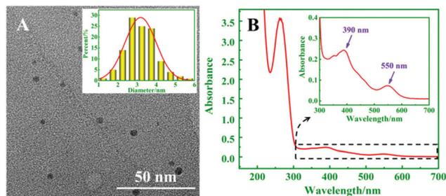
**Fig. 1** (A) TEM image of Ag NCs (inset: size distribution of Ag NCs). (B) UV-vis absorption spectrum of Ag NCs (inset: magnification of the UV-vis absorption spectrum in the wavelength range of 300–700 nm).
