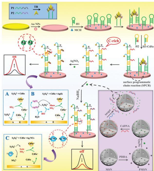
**Scheme 1** Schematic diagram of the “on-off” ECL biosensing platform for versatile detection of thrombin and miRNA-21 based on Ag(I) ion-accelerated and Ag NC-quenched ECL combined with molecular machine-triggered chain reaction and MSN double amplification.
