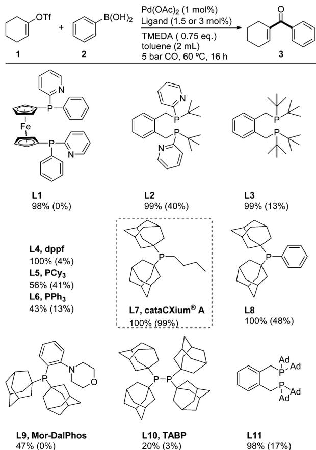
**Scheme 2** Pd-catalyzed synthesis of 1-cyclohexenyl phenyl ketone in the presence of different ligands. Reaction conditions: 0.5 mmol **1**, 1.2 eq. of **2**, 1.5 mol% for diphosphines, 3 mol% for monophosphines, in argon. Yields and conversions were determined by GC with *n*-hexadecane as standard, the values given within parentheses refer to the yields of **3** while the other values refer to the conversions of **1**.
