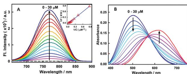
**Fig. 1** (A) Fluorescence spectra of  $15 \mu\text{M}$  styryl-11 with increasing concentration of insulin fibrils ( $0$ – $30 \mu\text{M}$ ) [ $\lambda_{\text{ex}} = 630$  nm]. Inset shows the double reciprocal plot ( $1/F$  vs.  $1/C$ ) and the solid line represents the fitting of the data points according to the  $1:1$  binding model. (B) Absorption spectra of  $15 \mu\text{M}$  styryl-11 with the increase in concentration of insulin fibrils ( $0$ – $30 \mu\text{M}$ ).
