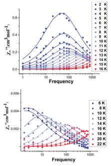
Fig. 3 Frequency dependent out-of-phase ac susceptibility signals for complex 1 (upper) and 3 (lower) in zero dc field. The solid lines correspond to the best fit.
