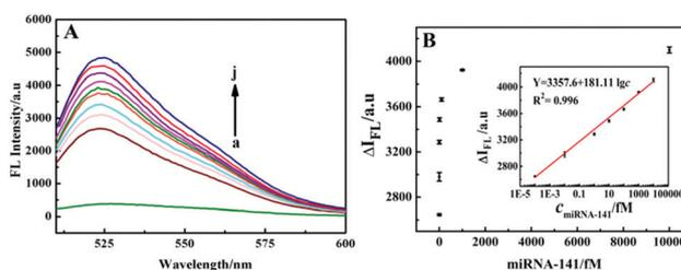
Fig. 4 (A) The fluorescence spectra of the SG I-based detection system in response to different concentrations of miRNA-141. (From a to j correspond to 0, 10<sup>-6</sup> fM, 10<sup>-4</sup> fM, 0.01 fM, 1.0 fM, 10 fM, 100 fM, 1.0 pM, 10 pM, and 100 pM.) (B) The relationship between the fluorescence signal ( $\Delta I_{FL}$ ) of SG I and the concentration of miRNA-141. Inset: Linear relationship between the fluorescence intensity and the logarithm of miRNA-141 concentration.
