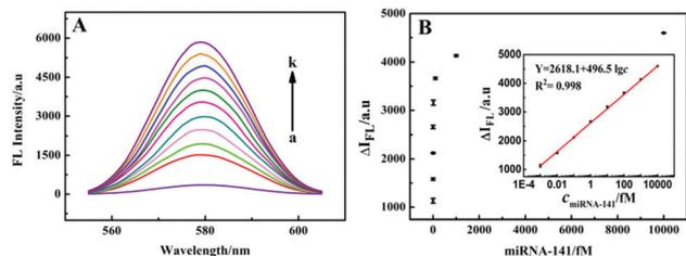
**Fig. 5** (A) The fluorescence spectra of the CdTe QD-based detection system in response to target miRNA-141 concentrations, (from a–k correspond to 0,  $10^{-3}$  fM, 0.01 fM, 0.1 fM, 1.0 fM, 10 fM, 100 fM, 1.0 pM, 10 pM, 100 pM, and 1.0 nM). (B) Relationship between the fluorescence signal ( $\Delta F_{FL}$ ) of CdTe QDs and miRNA-141 concentration. Inset: Linear relationship between the fluorescence intensity and the logarithm of miRNA-141 concentration.
