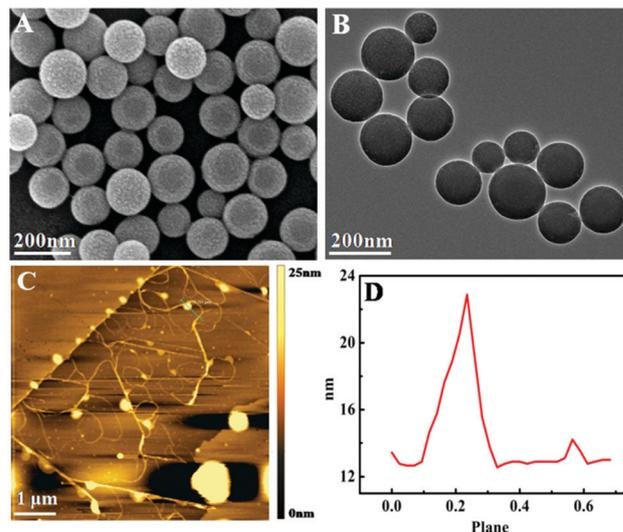
Fig. 3 (A) SEM image of SiO<sub>2</sub> microspheres; (B) TEM image of SiO<sub>2</sub> microspheres; (C) AFM image of SiO<sub>2</sub>-DNA hydrogel by HCR; and (D) height profile of SiO<sub>2</sub>-DNA hydrogel by HCR.
