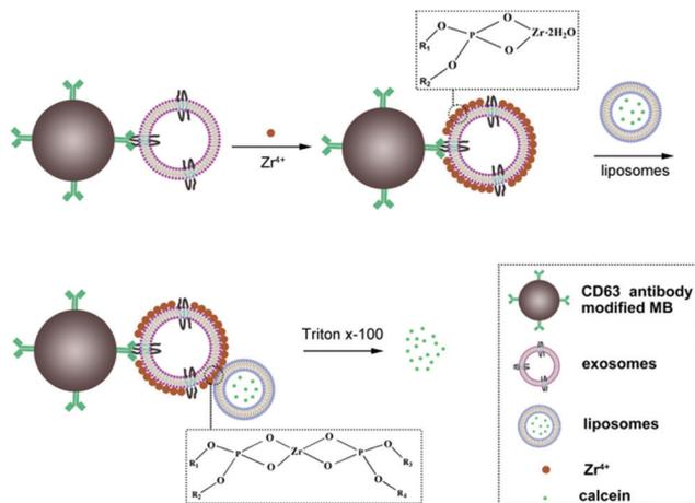
**Scheme 1** Working principle of the assay for the detection of exosomes based on phosphate– $Zr^{4+}$  coordination interaction and liposome-based signal amplification. In order to clearly display the exosome–zirconium–liposome sandwich structure, the diameter of MB, exosomes and liposomes doesn't represent real size contrast.
