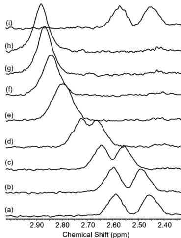
Fig. 6 Partial  $^1\text{H}$  NMR spectra of rotaxane **1** with: (a) 0 eq. of TFA, (b) 2 eq. of TFA, (c) 5 eq. of TFA, (d) 10 eq. of TFA, (e) 20 eq. of TFA, (f) 30 eq. of TFA, (g) 40 eq. of TFA, (h) 50 eq. of TFA, (i) 50 eq. of TFA + 50 eq. of  $\text{D}_5\text{-pyridine}$  ( $\text{CDCl}_3$ , 400 MHz, 298 K. Spectra Fourier transformed with a line broadening of 3 Hz).
