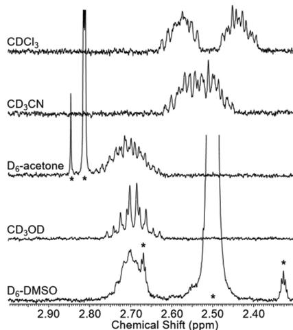
Fig. 5 Partial  $^1\text{H}$  NMR spectra of rotaxane **1** in various solvents (2.5 mM, 400 MHz, 298 K). Solvent peaks marked with asterisks.
