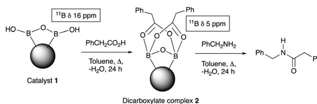
Scheme 1 Activation process of polymer catalyst **1**.
