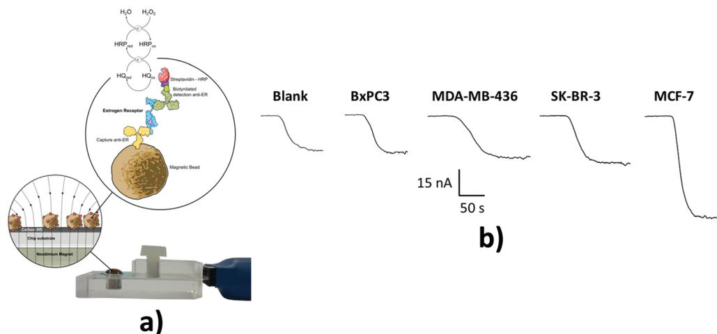
Fig. 13 (a) Schematic illustration of MB-based sandwich immunosensor developed for ER $\alpha$  determination. (b) Amperometric responses recorded in the absence (blank) and presence of 2.5  $\mu\text{g}$  of raw lysates from the corresponding cells. Reproduced and adapted from ref. 53 with permission.
