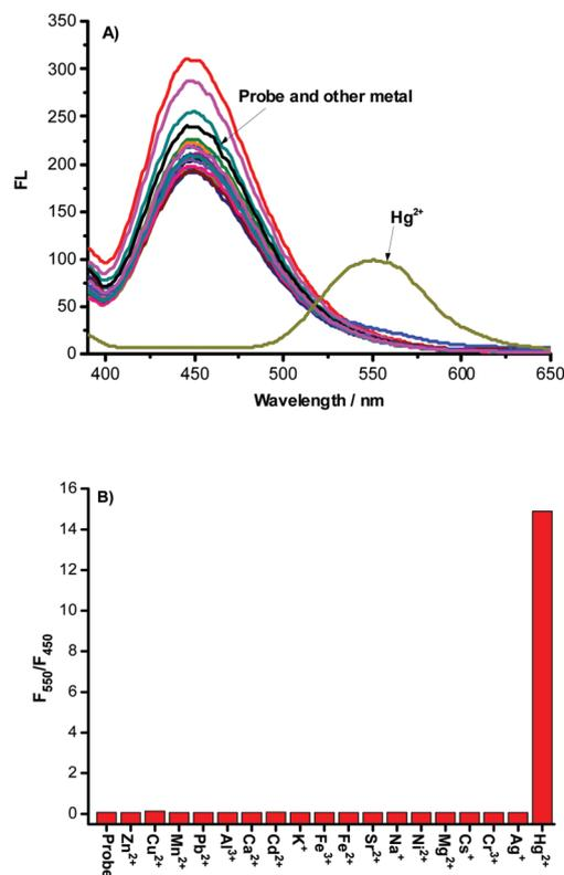
Fig. 2 (A) Fluorescence spectra of probe **NAP-PS** (10  $\mu\text{M}$ ) before and after the addition of 200  $\mu\text{M}$  different metal ions in HEPES buffer (1.0 mM, pH = 7.4),  $\lambda_{\text{ex}} = 380$  nm, slits: 3/5 nm; (B) fluorescence intensity ratios ( $F_{550}/F_{450}$ ) of probe **NAP-PS** (10  $\mu\text{M}$ ) before and after the addition of 200  $\mu\text{M}$  different metal ions in HEPES buffer (1.0 mM, pH = 7.4).
