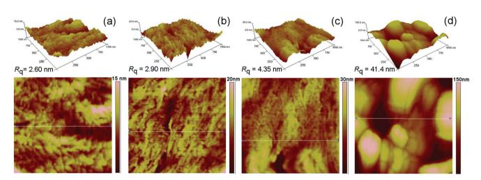
Fig. 5 Topographical changes after aminolysis and heparinization of model PLCL films: AFM images and height profiles of the pristine PLCL (a), Am-PLCL (30 min at 22 °C) (b), PA-Hep-PLCL (15 h) (c) and CL-Hep-PLCL (6 h) coated surfaces. Scan size:  $1 \times 1 \,\mu\text{m}^2$ .
