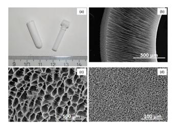
Typical morphological features of PLCL capsules: (a) a digital camera image of the capsule (left) along with a Teflon bar (right) used to block the core of the capsule during implantation. SEM images of the capsule's cross section (b), outer surface (c), and inner surface (d).
