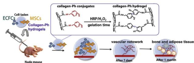
**Fig. 10** Schematic illustration of fabricating collagen-Ph hydrogel and *in vivo* experiment. Collagen was conjugated with tyramine and the injectable hydrogel containing ECFs and MSCs formed in the presence of HRP/H<sub>2</sub>O<sub>2</sub>. Cell-loaded hydrogels could form vascular networks after 7 days and promote adipose and bone-like tissue formation. Reproduced with permission from *Acta Biomater.*, 2015, 27, 151–168. Copyright 2015 Elsevier.<sup>131</sup>
