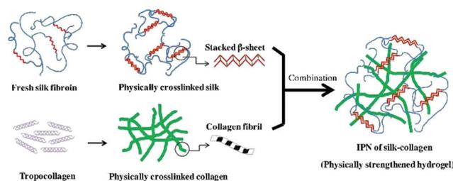
**Fig. 4** The schematic illustration of ultrasonic induced gelation of fibroin/collagen IPNs. Silk fibroin solution was placed in an ultrasound device for inducing  $\beta$ -sheet formation, and the ultrasonicated solution was added to the collagen solution. The mixed solution was aliquoted into a mold and incubated at 37 °C for complete gelation. Reproduced with permission from *Acta Biomater.*, 2018, 69, 218–233. Copyright 2018 Elsevier.<sup>63</sup>
