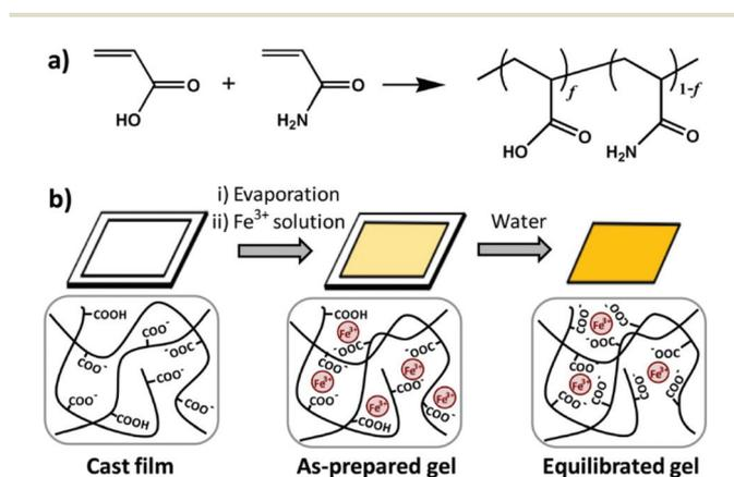
**Fig. 7** Diagrams of synthesis of copolymers (a) and physical crosslinked hydrogels (b). Hydrogels were formed by carboxyl-Fe<sup>3+</sup> coordination. The dynamic nature of coordination bonds was rate dependent and the mechanical performance of hydrogels could be tuned by controlling the composition of copolymers, concentration of metallic ions, and pH values of solutions. Reproduced with permission from *Macromolecules*, 2016, **49**, 9637–9646. Copyright 2016 ACS.<sup>83</sup>
