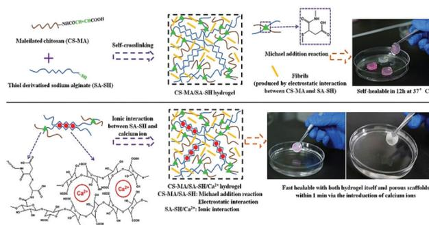
**Fig. 2** Schematic illustration of the fibrils-reinforced polysaccharide-based composite hydrogels. The hydrogels were generated by self-crosslinking of CS-MA and SA-SH. The ionic interaction between CS-MA and SA-SH was able to improve mechanical properties of hydrogels. Reproduced with permission from *Compos. Sci. Technol.*, 2018, 156, 238–246. Copyright 2018 Elsevier.<sup>54</sup>
