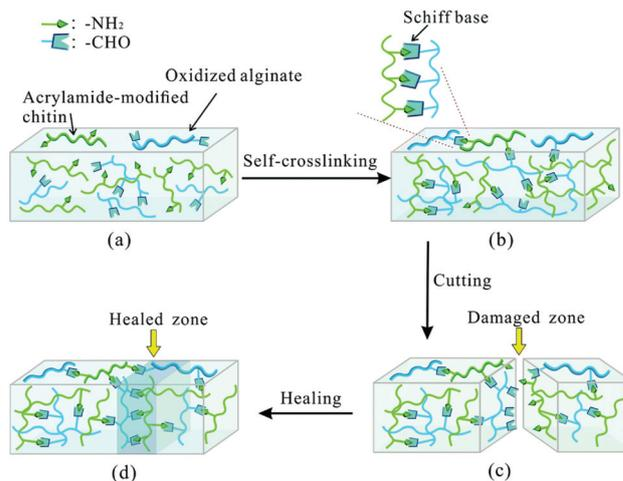
**Fig. 12** Schematic illustration of Schiff base formation and self-healing process. The self-crosslinked hydrogel was synthesized *via* Schiff base linkage between the amino group of acrylamide-modified chitin (AMC) and the dialdehyde group (ADA) of oxidized alginate. The self-healing capability relied on the molar ratio of AMC and ADA as well as pH. Reproduced with permission from *Soft Matter*, 2015, 11, 3971–3976. Copyright 2015 RSC.<sup>137</sup>
