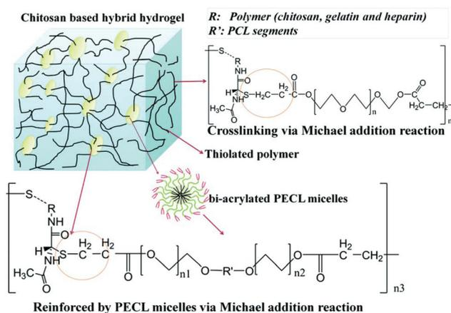
**Fig. 14** Schematic illustration of Michael addition of chitosan-based hydrogels cross-linked with PECL micelles. Chitosan, gelatin and heparin were thiolated and crosslinked with PEGDA and bi-acrylated PECL micelles at different molar ratios. Reproduced with permission from *J. Mater. Chem. B*, 2017, 5, 961–971. Copyright 2017 RSC.<sup>141</sup>
