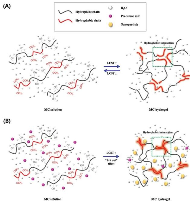
**Fig. 3** The sol-to-gel transition process of MC, (A) pure MC solution and (B) MC solution with salt. As the temperature increases, hydrogen bonds are broken, which results in hydrogel formation. Addition of salts to the MC solution destroys hydrogen bonds and reduces the sol-gel transition temperature and time. Reproduced with permission from *Carbohydr. Polym.*, 2017, 15, 775–783. Copyright 2017 Elsevier.<sup>58</sup>
