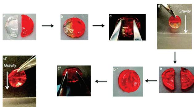
**Fig. 13** Schematic illustration of self-healing behaviour. Two previously cut pieces of hydrogels (a) were placed in contact for 2 h (b) and the repaired gels were stretched with tweezers (c and c'); the healed gels were suspended under gravity (d and d'). When the gel was self-healed for 24 h, the hydrogel was cut again (e). Reproduced with permission from *Soft Matter*, 2015, 11, 6152–6161. Copyright 2015 RSC.<sup>34</sup>
