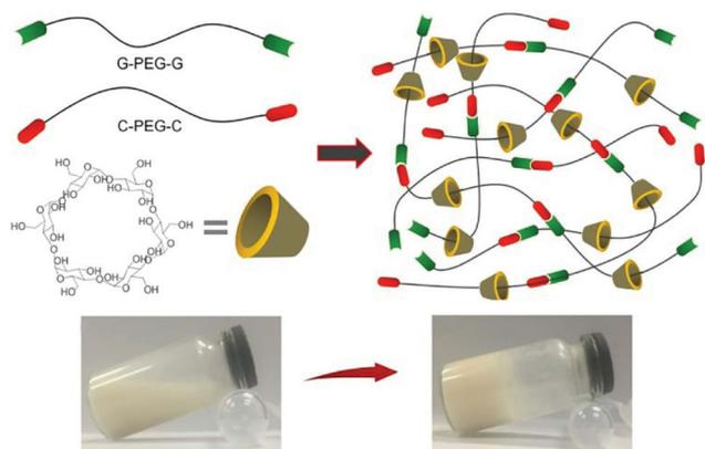
**Fig. 8** Synthesis of supramolecular hydrogels by host–guest inclusion between guanine/cytosine (G/C)-terminated PEG and  $\alpha$ -cyclodextrin. The G–C base pairing acts as additional network junctions and enhances the hydrogel mechanical properties. These hydrogels also exhibit excellent cytocompatibility and temperature-responsivity. Reproduced with permission from *Mater. Sci. Eng., C*, 2018, **82**, 25–28. Copyright 2016 Elsevier.<sup>94</sup>
