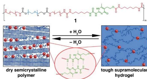
**Fig. 6** The PEG-UPy copolymers with multiblock architectures and self-complementary quadruple H-bonding interaction between 2 UPy segments. The descriptive morphology of dry semicrystalline polymer and a reversible transition to hydrogel. Reproduced with permission from *J. Am. Chem. Soc.*, 2014, 136, 6969–6977. Copyright 2014 ACS.<sup>71</sup>
