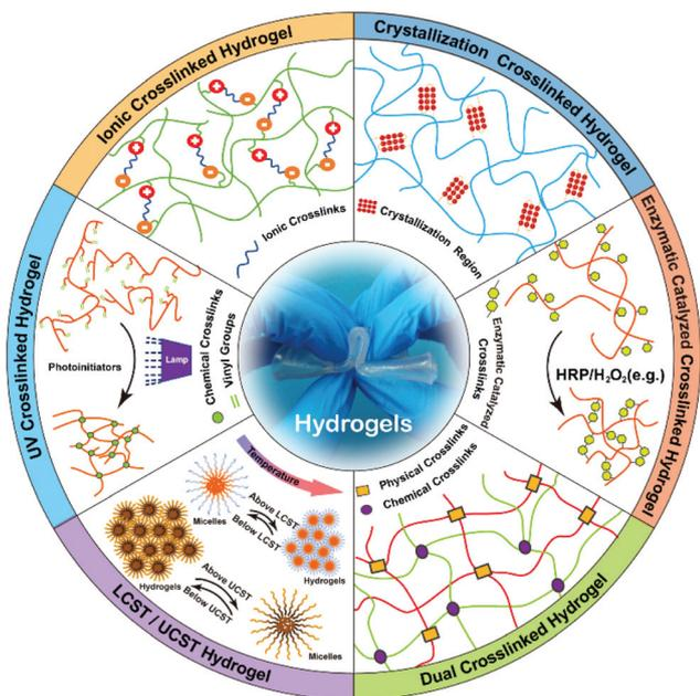
**Fig. 1** Crosslinking strategies for hydrogel construction. In this diagram, the most widely used crosslinking methods are presented, including physical crosslinking, such as ionic crosslink, LCST/UCST induced hydrogel formation, crystallization induced hydrogel formation and chemical crosslinking, such as UV-induced crosslink and Enzyme catalyzed crosslink.
