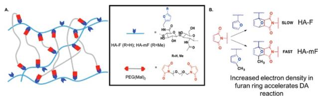
**Fig. 11** Schematic illustration of Diels–Alder (DA) reaction. When the furan group is replaced by methylfuran, DA reaction accelerates and hydrogels can be synthesized efficiently at pH 7.4 since the methylfuran group provided a more electron-rich diene. Reproduced with permission from *Biomacromolecules*, 2018, 19, 926–935. Copyright 2018 ACS.<sup>134</sup>
