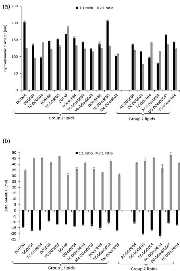
**Fig. 2** (a) The apparent hydrodynamic size (nm) and (b) zeta potential (mV) of LDs prepared from vesicles of the cationic lipids in combination with either DOPE or (\*) DOPC and ctDNA at L : D charge ratios of either 2 : 1 (grey bars) or 1 : 1 (black bars), respectively, and a ctDNA concentration of  $1 \mu\text{g mL}^{-1}$ . All measurements were performed in triplicate at  $298 \pm 0.1$  K on the day of preparation and are shown as the mean value  $\pm$  standard deviation.
