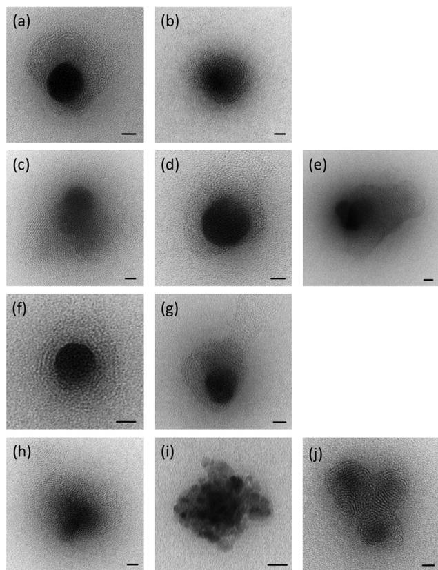
**Fig. 4** Transmission electron microscopy of LD complexes (lipoplexes prepared using ctDNA at a cationic lipid : DNA charge ratio of 2 : 1 made with (a) DODEG4; (b) DOesDEG4; (c) TC-DODEG4; (d) TC-DOesDEG4; (e) Me-DOesDEG3; (f) DOSEG3; (g) DOesSEG3; (h) TC-DOSEG3; (i) TC-DOesSEG3; (j) Me-DOesSEG3. Size bar = 20 nm.
