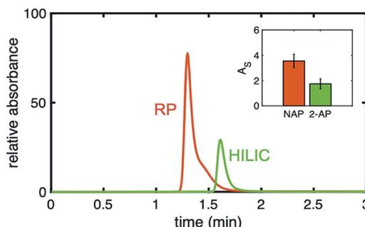
**Fig. 7** Chromatogram of naphthol (red, 30% ACN) and 2-AP (green, 70% ACN) acquired on the same phenyl–butyl gradient column but under two different mobile phase compositions. Inset: The asymmetry factors of naphthol at 30% ACN (red) and 2-AP at 70% ACN (green) on the same phenyl–butyl gradient. Column: Error bars represent  $n = 3$  columns.
