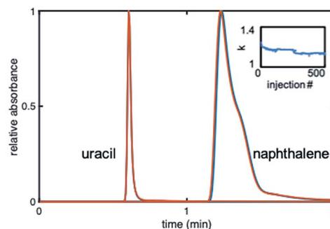
Fig. 5 Chromatograms depicting uracil and naphthalene at injections #50 (blue) and #500 (red) at 40% ACN on the gradient phenyl-butyl columns. Inset: The retention factor of naphthalene *versus* injection number.
