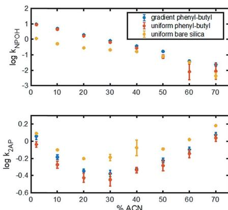
Fig. 4 Correlation between  $\log k$  and % ACN for naphthol (top) and 2-AP (bottom) for phenyl-butyl gradient (blue), phenyl-butyl uniform (red), and bare silica uniform (yellow) columns. Error bars represent  $n = 3$  columns.
