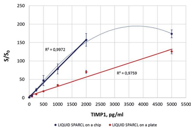
**Fig. 3** Quantitative measurement of TIMP1 on the chip using liquid reagents and off-chip preparation of reactions. Here and further, the error bars designate the standard deviation; number of replicates  $n = 3$ .
