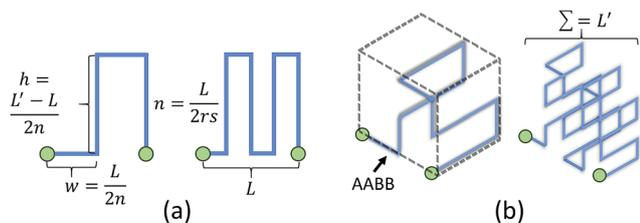
Fig. 4 Two iterations of 2D and 3D square curves. (a) The total channel length  $L'$  of a 2D square curve is computed by equation:  $L' = L + 2hn$ . (b) The total channel length  $L'$  of a 3D square curve is computed by equation:  $L' = (1 + 2n)L + 4hn^2$ .
