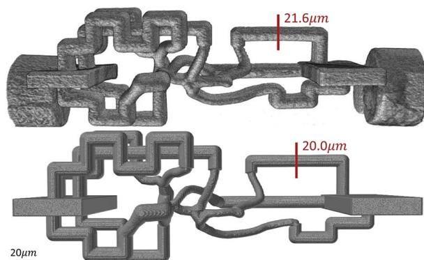
Fig. 9 3D volume rendering of a fabricated microvascular network (top) and its digital mask (bottom) shows a close agreement in overall architecture and channel diameters between them. SB = 20  $\mu\text{m}$ .
