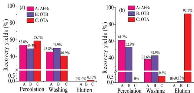
**Fig. 7** Cross-reactivity of three toxins on the PMAA monolithic column targeting OTA; (a) ssDNA control monolith; (b) PMAA monolith. A: aflatoxin B1, B: ochratoxin B, C: ochratoxin A. The concentrations of OTA, OTB and AFB<sub>1</sub> were both  $10 \text{ ng mL}^{-1}$ .
