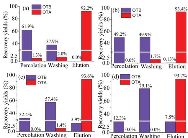
**Fig. 5** Recoveries of OTA and OTB on affinity monoliths with different POSS-MA: (a) 2.5% POSS-MA; (b) 5.0% POSS-MA; (c) 7.5% POSS-MA; (d) PMAA monolithic column. The concentrations of OTA and OTB were both 10 ng mL<sup>-1</sup>.
