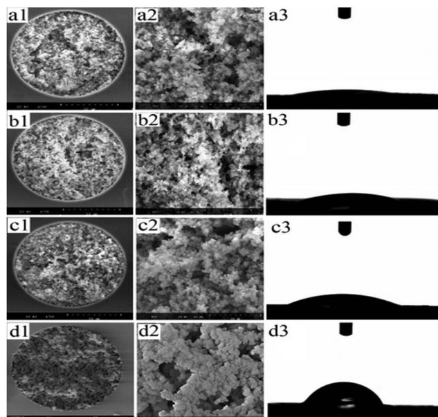
**Fig. 1** SEM images of different monolithic columns and the contact angles of water on the flat sheets of monolithic surfaces: (a) PMAA column with 2.5% POSS-MA; (b) PMAA column with 5.0% POSS-MA; (c) PMAA column with 7.5% POSS-MA. (d) PMAA column; magnification times: (a1–d1)  $\times 700$ , (a2–d2)  $\times 2000$ .
