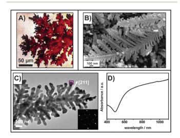
Fig. 1 (A) Optical image of dendritic microstructures prepared by pulsed-current deposition of copper. <sup>42</sup> (B) SEM image of silver dendrites on a copper substrate prepared by galvanic replacement. <sup>45</sup> (C) TEM image gold nanodendrites prepared using a poly(ionic liquid) method. <sup>50</sup> (D) absorbance spectrum of the gold nanodendrites. Reprinted and adapted from ref. 42, 50, and 45. Copyrights Elsevier 1998 and 2017, and The Royal Society of Chemistry respectively.
