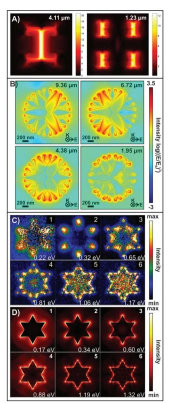
Fig. 5 EM field distributions for (A) an H-tree fractal, 87 and (B) a threebranched fourth-order generation dendritic fractals.<sup>59</sup> (C) Experimental EELS maps and (D) corresponding calculated EM field maps for a firstorder generation Koch fractal.86 Reproduced and adapted with permission from ref. 87, 59, and 86. Copyrights 2013 IOP Publishing and 2017 American Chemical Society respectively.
