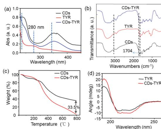
**Fig. 2** (a) UV-Vis spectra of CDs, TYR and CDs–TYR, respectively; (b) FT-IR spectra of CDs, TYR and CDs–TYR; (c) TGA curves of CDs and CDs–TYR; (d) CD spectra of TYR before (black line) and after (red line) the conjugation with CDs.
