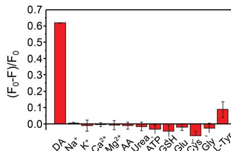
**Fig. 4** Relative fluorescence decrement  $((F_0 - F)/F_0)$  of the bioprobe ( $15\ \mu\text{g mL}^{-1}$ ) in the presence of different interfering substances.  $F_0$ : Fluorescence intensity of the blank,  $F$ : fluorescence intensity of the bioprobe upon the addition of the inspected species. Dopamine: 10  $\mu\text{M}$ ,  $\text{Na}^+/\text{K}^+$ : 1 mM, *L*-Tyr: 10  $\mu\text{M}$ , other substances: 100  $\mu\text{M}$ .
