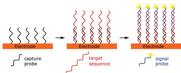
Fig. 2 Schematic representation of a sandwich sensor.
