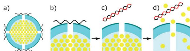
**Fig. 4** Mechanism of miRNA detection using mesoporous silica. (a) Mesoporous silica is loaded with electroactive signalling molecules. (b) The pores of the silica are capped with miRNA capture probes. (c) Complementary binding leads to dissociation from the pores. (d) The electroactive molecules escape the silica to be detected on an electrode.
