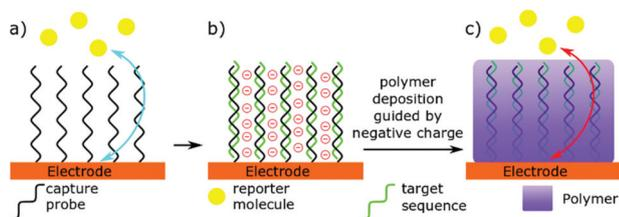
**Fig. 3** Principle of an impedance-based polymer film biosensor. (a) In absence of microRNA target, the electrode can easily detect reporter molecules. (b) Complementary binding brings a negative charge to the surface. (c) Polymer deposition inhibits charge transfer.
