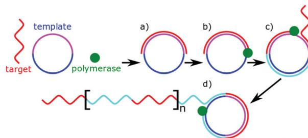
**Fig. 5** General principle of rolling circle amplification (RCA). (a) Target complementary binds to circular template. (b) The polymerase uses target sequence as a primer. (c) The polymerase displaces the target as it processes around the template. (d) The result is tandem repeats of the target sequence with a designed secondary sequence.
