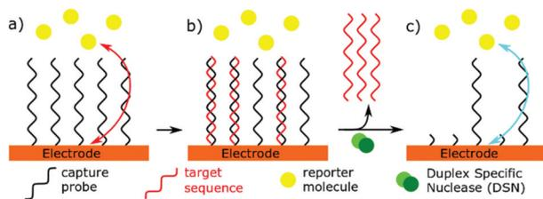
**Fig. 6** The use of duplex specific nuclease in biosensing. (a) Electron transfer is hindered by a surface concentration of capture probes. (b) Complementary binding of the target sequence allows duplex specific nuclease to selectively remove capture probes. (c) Electron transfer is easier as a result.
