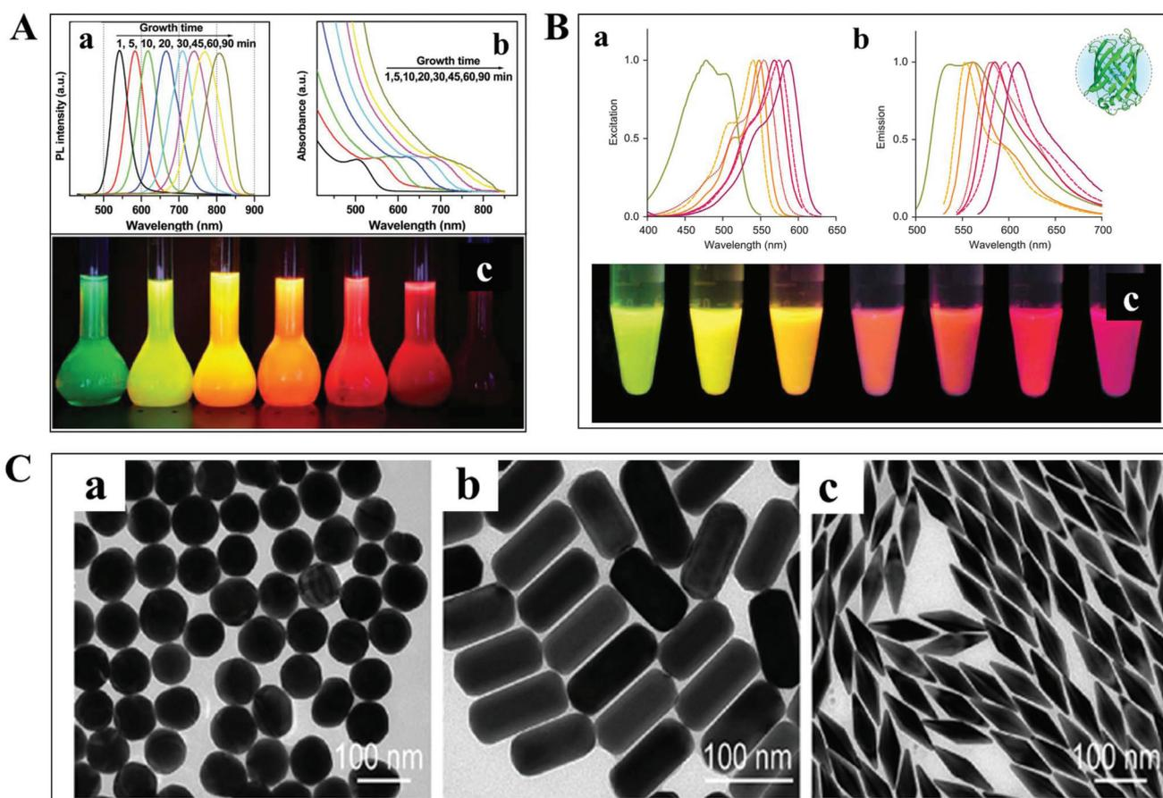
**Fig. 3** (A) Fluorescence emission spectra (a), UV-vis absorption spectra (b) and photographs (c) under ultraviolet light of cadmium telluride QDs at different reaction times.<sup>36</sup> (B) Excitation (a), emission spectra (b), and photographs (c) of different fluorescent proteins under ultraviolet light excitation.<sup>38</sup> (C) TEM images of GNPs with different shapes.<sup>41</sup>
