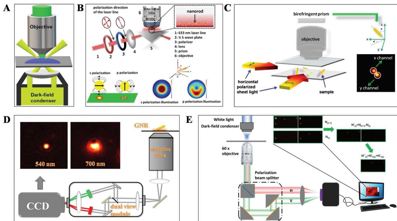
Fig. 2 Schematic diagram of (A) DFM, (B) total internal reflection scattering microscopy (TIRSM),<sup>32</sup> (C) planar illumination microscopy,<sup>33</sup> (D) dual-wavelength upright DFM,<sup>34</sup> and (E) DFM with a polarization-resolved dual-channel imaging module.<sup>35</sup>
