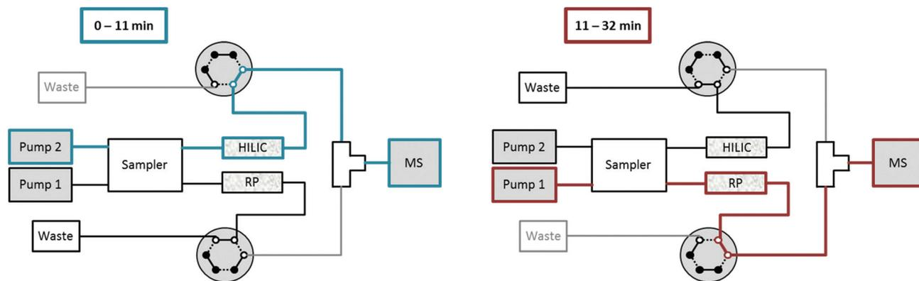
**Fig. 1** Dual setup for HILIC-RP MS with two pumps, an autosampler with two independent flow-paths and two 2-position-6-port valves. From 0–11 min HILIC elution of metabolites is carried out and directed into the MS, followed by RP elution of lipids which are injected after 10 min. During column re-equilibration of each column, the flow is directed to a waste bottle allowing for stable conditions during elution of the other column.
