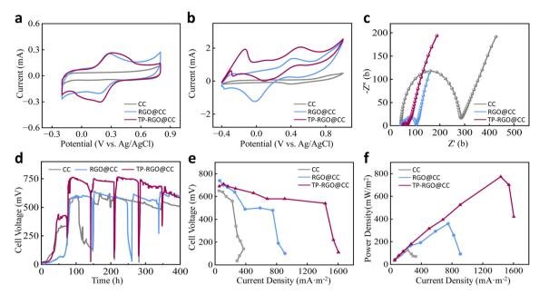
Fig. 3 (a) The cyclic voltammetry curve CV of the material was scanned in PBS solution; (b) the CV curve of the material in MFCs; (c) Nyquist plots of different anodes; (d) time course of voltage output; (e) and (f) the polarization and power density curves as a function of the current density of MFCs with different anodes.
