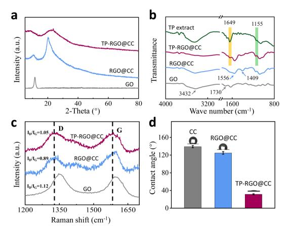
(a) XRD spectra; (b) FTIR spectra; (c) Raman spectra and (d) contact angles of CC, RGO@CC, TP-RGO@CC anodes
