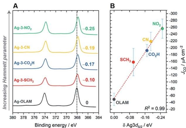
Fig. 4 (A) X-ray photoelectron spectra for Ag-OLAM and hybrid catalysts bearing octyl tail-groups, showing shifts in the Ag 3d<sub>5/2</sub> peaks. (B) Correlation of these XPS shifts with the CO<sub>2</sub>RR performance, described by  $J_{CO}$ , where larger shifts in the Ag XPS peaks are accompanied by a greater improvement in the performance.
