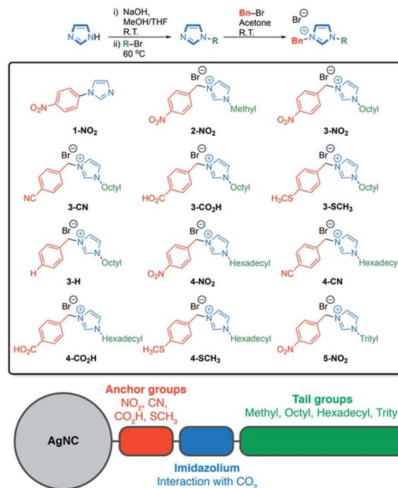
Scheme 1 Synthetic route to asymmetrically disubstituted imidazolium compounds and a schematic overview of the hybrid AgNC catalysts. 1-NO<sub>2</sub> was instead prepared by an Ullmann-type reaction. 2-NO<sub>2</sub> was prepared directly from 1-methyl-imidazole. Abbreviations: Bn = benzyl group; methyl = CH<sub>3</sub>; octyl = *n*-C<sub>8</sub>H<sub>17</sub>; hexadecyl = *n*-C<sub>16</sub>H<sub>33</sub>; trityl = C(C<sub>6</sub>H<sub>5</sub>)<sub>3</sub>.
