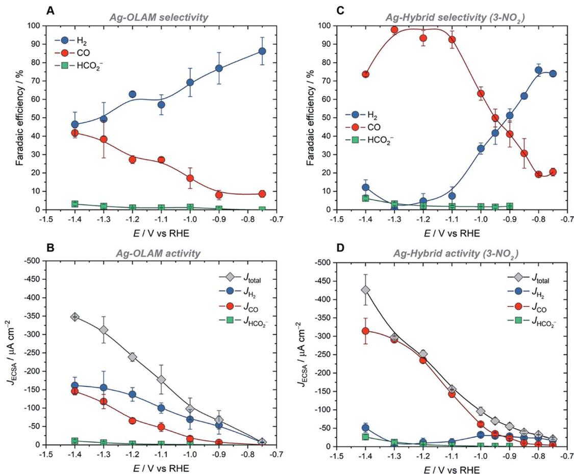
Fig. 3 Performance of **Ag-OLAM** and **Ag-3-NO<sub>2</sub>** CO<sub>2</sub>RR catalysts at variable applied potential, showing: (A) Faradaic efficiencies of products and (B) total and partial current densities measured for **Ag-OLAM**; (C) Faradaic efficiencies of products and (D) total and partial current densities measured for **Ag-3-NO<sub>2</sub>**. Error bars represent standard deviation based on at least three independent measurements.
