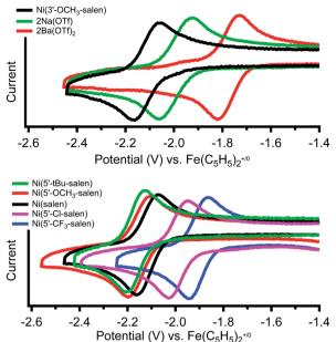
Fig. 2 Cyclic voltammograms of the reversible Ni(II/I) redox couples of (top) Ni(3'-OCH $_3$ -salen) and 2M (M = Na $^+$ , Ba $^{2+}$ ) and (bottom) Ni(5'-R-salen) where (R = CF $_3$ , Cl, tBu, OCH $_3$ ) in 0.1 M tetrabutylammonium hexafluorophosphate in dimethylformamide under N $_2$  at a scan rate of 1 V s $^{-1}$ .
