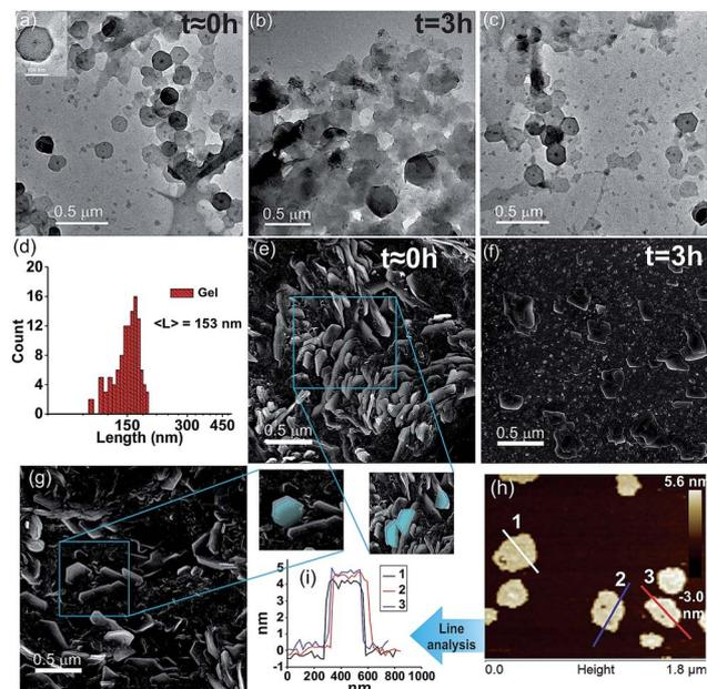
**Fig. 2** TEM images of (a) **C18A-Fc-NMe<sub>2</sub>** for  $t \approx 0$  h (inset: enlarged view), (b)  $t = 3$  h sol, and (c) refueled gel (4 mM **Fc-NMe<sub>2</sub>**). (d) Histogram of hexagon dimensions from the TEM results at  $t \approx 0$  h. SEM images (e) at  $t \approx 0$  h with blue traces showing the hexagonal structures, (f)  $t = 3$  h sol, (g) refueled gel (5 min), and (h) AFM image at  $t \approx 0$  h and (i) the corresponding height profiles.
