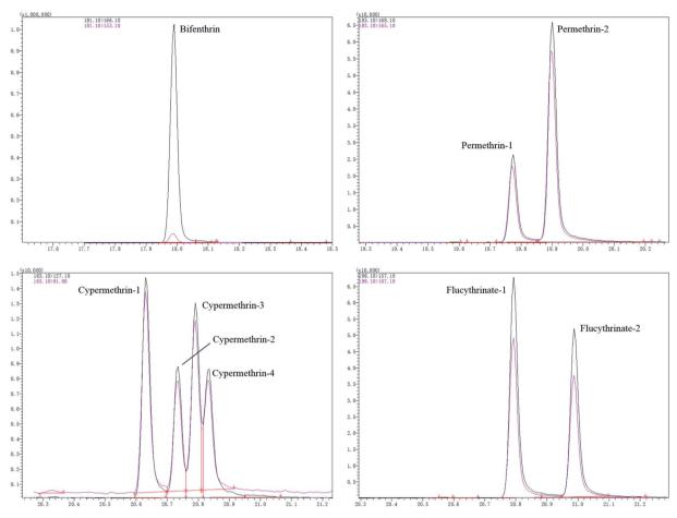
Fig. 4 Extracted total ion chromatograms obtained by the proposed method for pyrethroids from a real tea sample (Sichuan Maofeng) spiked at  $10 \mu g L^{-1}$ .
