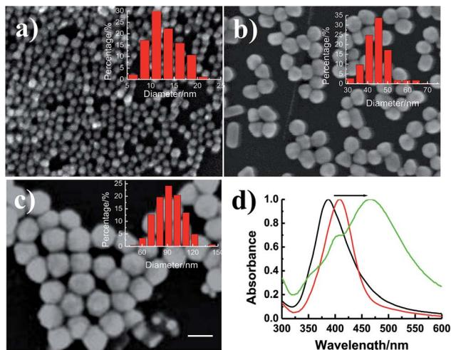
**Fig. 1** SEM images and corresponding size distributions of AgNPs. The average particle sizes are 13.02 nm (a), 45.21 nm (b) and 92.18 nm (c). The total numbers of particles counted for the histograms are more than 100. Scale bar: 100 nm. (d) Extinction spectra of AgNPs with the size of 13.02 nm (black), 45.21 nm (red) and 92.18 nm (green).
