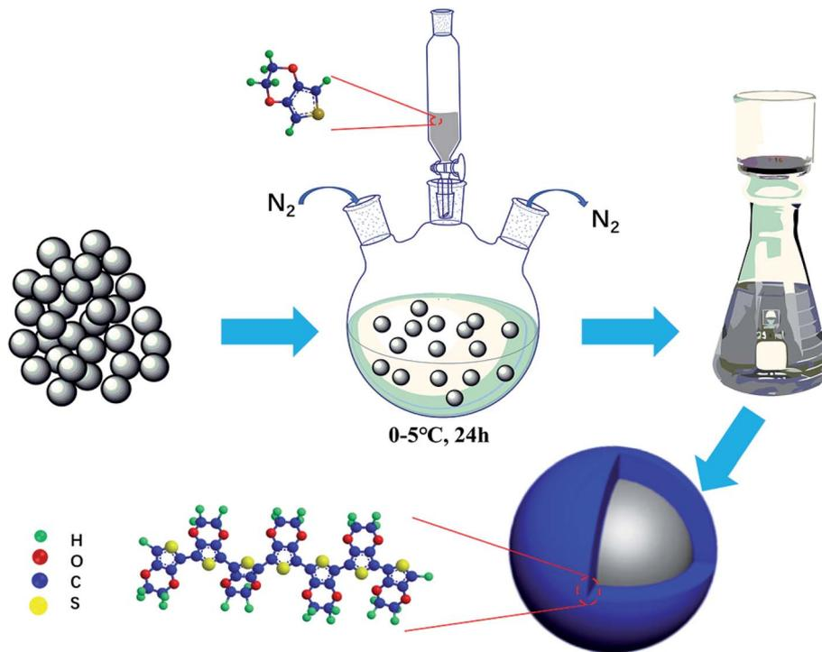
Fig. 1 Coating process of PEDOT on LNMO and the facial structure for PEDOT-coated LNMO.
