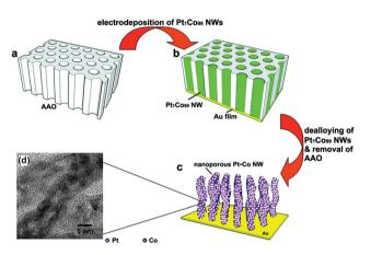
Fig. 9 (a-c) Schematic illustrations of the fabrication process of nanoporous Pt-Co alloy NWs. (d) High-resolution TEM micrographs of the as-prepared nanoporous Pt-Co alloy NWs. Adapted with permission from ref. 118. Copyright 2009, American Chemical Society.
