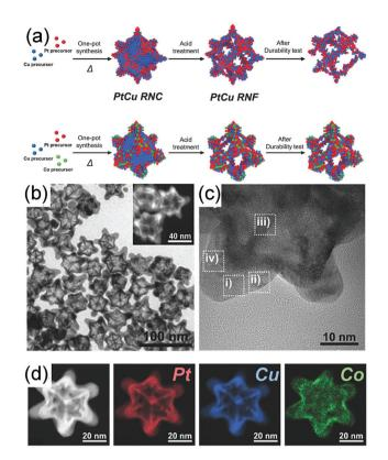
Fig. 11 (a) Schematic illustration of the formation process of PtCu RNC, PtCu RNF, Co-PtCu RNC, and Co-PtCu RNF. (b)TEM and (c) HRTEM images and (d) HAADF-STEM image and corresponding EDS elemental mapping analysis of Co-PtCu RNF. Adapted with permission from ref. 24. Copyright 2018, Wiley-VCH.
