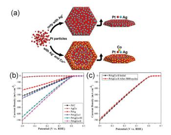
Fig. 20 (a) Schematic illustration of PtAg and PtAgCo nanosheets. (b) Polarization curves for PtAq, AqCo, and PtAqCo nanostructures prepared at different molar ratios: (PtAg) 0.01:0.01, (AgCo) 0.01:0.01, (PtAgCo-I) 0.01:0.01:0.005, (PtAgCo-II) 0.01:0.01:0.01, and (PtAgCo-III) 0.01:0.01:0.015 in 0.5 M H<sub>2</sub>SO<sub>4</sub>. (c) Durability tests of PtAgCo-II samples. Adapted with permission from ref. 224. Copyright 2017, American Chemical Society
