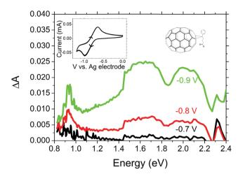
Fig. 4 Electrochemically induced absorbance in  $PC_{71}BM$  with cyclic voltammogram and chemical structure shown in the inset.
