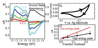
Fig. 3 (a) Electrochemically induced change of absorbance in PTB7 film at different voltages applied to the ITO electrode (left axis) and its ground state absorbance (right axis). (b) Cyclic voltammogram for PTB7 with direction of scan shown with arrow heads. (c) Induced absorbance at the low energy peak (around 1.1 eV) and the high energy peak (around 1.65 eV) vs. the fraction of chromophores oxidized, which was obtained from eqn (1).
