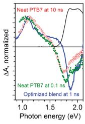
**Fig. 2** Transient absorption spectra of neat PTB7 film after excitation at 2.3 eV and of optimized PTB7:PC $_{71}$ BM blend normalized at the photo-induced absorption maximum around 1.1 eV. Black line shows ground state absorption spectrum of neat PTB7 film.
