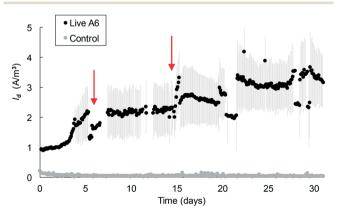
Fig. 5 Average current density measured in MECs with a pure A6 culture under stirring conditions. Marks show the mean and lines show the standard error. A representative control MEC containing dead A6 is shown in the figure. Arrows represent the times of headspace flushing and injection of an 80% N2 and 20% CO2 gas mixture.
