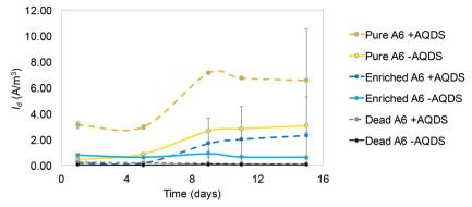
Fig. 2 Average current density measured in MECs containing live pure A6 and A6 enrichment cultures, with and without AQDS, and dead cultures with and without AQDS (Vapp 0.7 V). The points show the mean and the bars the standard error. Notice that the addition of AQDS has a greater effect on the pure A6 cultures than on A6 enrichment cultures, and no significant effect of AQDS on current production is found in dead cultures.
