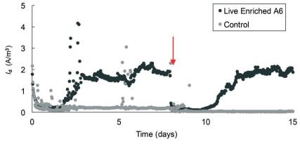
Fig. 6 Average current density measured in MECs containing an A6 enrichment culture. The arrow represents the point of headspace flushing and injection of an 80% N<sub>2</sub> and 20% CO<sub>2</sub> gas mixture.
