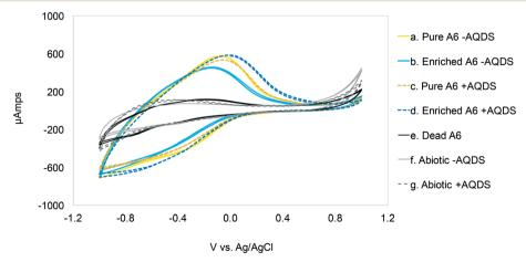
Fig. 1 Cyclic voltammetry scans (1 mV per second) for MECs with and without Acidimicrobiaceae sp. A6, and with (+AQDS) and without (-AQDS) AQDS. Optimal  $V_{app}$ :  $\simeq 0.03 \pm 0.025$  V vs. Ag/AgCl for cultures with AQDS and  $-0.11 \pm 0.035$  V vs. Ag/AgCl for MECs without AQDS.
