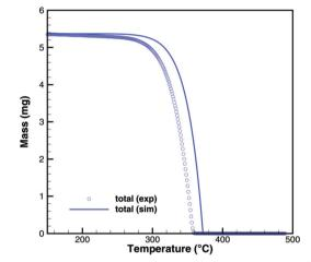
Fig. 14  $\,$  TG data of cyanuric acid (cylinder crucible, 2  $\,$  K  $\,$  min $^{-1}$ ) with simulated composition of the mixture.
