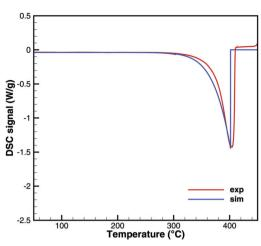
Fig. 13 DSC data of cyanuric acid (cylinder crucible).
