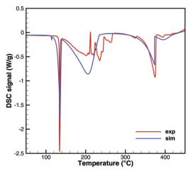
Fig. 20 DSC data of urea (cylinder crucible)
