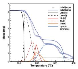
Fig. 21 TG data of urea (cylinder crucible, 2 K min<sup>-1</sup>) with simulated composition of the mixture
