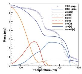
Fig.  $16~{\rm TG}$  data of triuret (cylinder crucible,  $2~{\rm K~min}^{-1}$ ) with simulated composition of the mixture.
