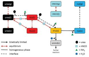
Fig. 12 Proposed reaction scheme of urea decomposition.
