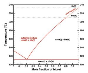
Fig. 2 Phase diagram of a eutectic mixture of urea and biuret.
