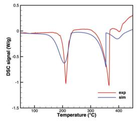
Fig. 15 DSC data of triuret (cylinder crucible).
