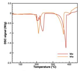
Fig. 7 Experimental DSC data for decomposition of biuret and triuret.
