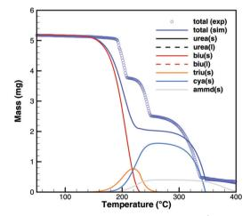
Fig. 18  $\,$  TG data of biuret (cylinder crucible, 2 K  $\,$  min $^{-1}$ ) with simulated composition of the mixture.
