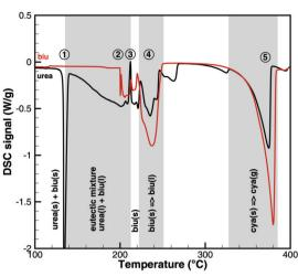
Fig. 3 Qualitative comparison of DSC signals for urea and biuret decomposition (1 – melting of urea, 2 – melting of biuret in a eutectic mixture, 3 – urea disappears, 4 – melting of biuret, and 5 – sublimation of cyanuric
