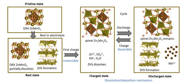
Schematic of the energy storage mechanism for the ZnMnO<sub>2</sub> DRX cathode in an aqueous ZIB.
