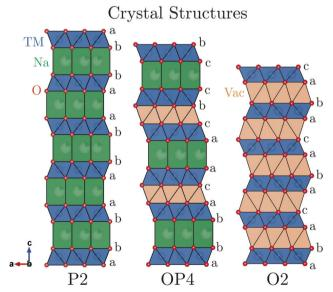
Fig. 1 The P2, OP4, and O2 crystal structures are shown projected parallel to the layers showing the stacking sequence.
