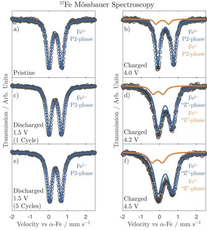
Fig. 7 <sup>57</sup>Fe-Mössbauer spectroscopy spectra at various states of charge with blue lines representing a Fe<sup>3+</sup> doublet fit, orange lines representing a Fe<sup>4+</sup> doublet fit, and the black line representing the total fit.
