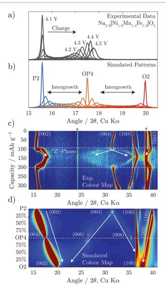
Fig. 6 Diffraction patterns are simulated using FAULTS for intergrowth structures composed of P2 and OP4, and OP4 and O2. These are plotted overlaid in (b) and over a wider  $2\theta$  range in (d) as a colour map. Experimental data for  $Na_{2/3}[Ni_{1/6}Mn_{1/2}Fe_{1/3}]O_2$  (also presented in Fig. 3b) is replotted in (a and c) for comparison to the simulations.
