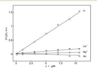
Fig. 5 Observed linear calibration curves of normalized fluorescence at 406 nm as a function of concentration of different cations for 18C6  $(\lambda_{excitation} = 346 \text{ nm}).$
