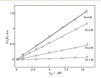
Fig. 8 Observed linear calibration curves of normalized fluorescence response of nanospheres based on **18C6** to the potassium cation at different sodium background levels.
