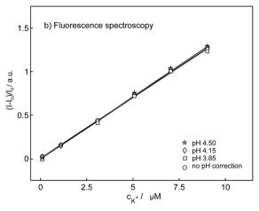
Fig. 9 (a) Potentiometric response of the potassium selective sensor to the changes in concentration of  $H^+$  at fixed concentration of potassium 1 mM and (b) observed linear calibration curves from the normalized fluorescence spectra as a function of potassium concentration at different pH.
