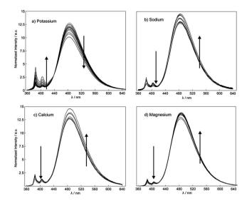
Fig. 6 Effect of the addition of (a) potassium, (b) sodium, (c) calcium and (d) magnesium on the fluorescence emission behavior of K<sup>+</sup> selective nanospheres ( $\lambda_{\text{excitation}} = 346 \text{ nm}$ ) in the concentration range  $10^{-6}$  to  $10^{-1}$  M.
