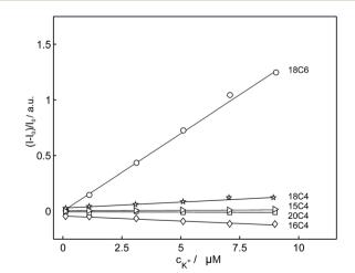
Fig. 4 Observed linear calibration curves of normalized fluorescence at 406 nm as a function of potassium concentration for different macrocyclic compounds (15C4, 16C4, 18C4, 18C6, 20C4) in exhaustive fluorescence mode ( $\lambda_{\text{excitation}} = 346 \text{ nm}$ ).
