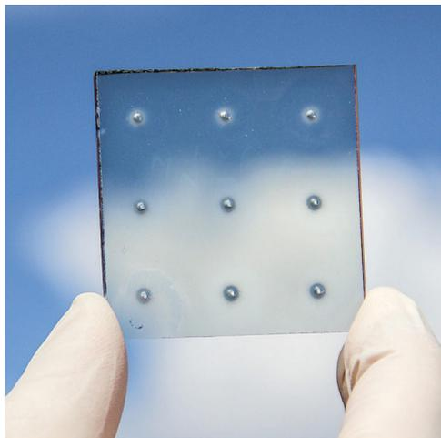
Fig. 27 Electropolymerized poly(3,4-ethylenedioxythiophene) on an FTO substrate.
