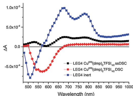
**Fig. 8** Photoinduced absorption spectra of LEG4-sensitized TiO<sub>2</sub> photoanodes (blue) as well as in contact with copper phenanthroline complexes in liquid junction (red) and solid-state (black) DSCs. Reproduced from ref. 107 with permission from the Royal Society of Chemistry.
