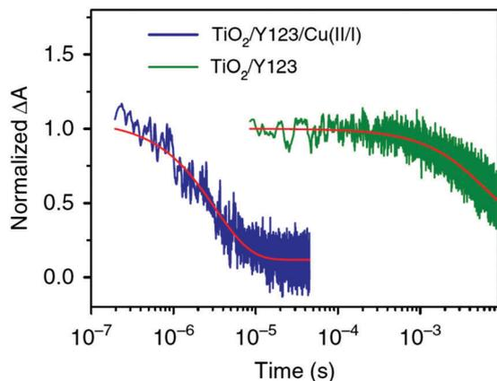
Fig. 9 Transient absorption spectra of **Y123**-sensitized photoanodes inert (green) and in contact with the solid  $\text{Cu}^{\text{II/I}}(\text{tmby})_2$  hole transport material. Reproduced from ref. 87 with permission from the Nature publishing group.
