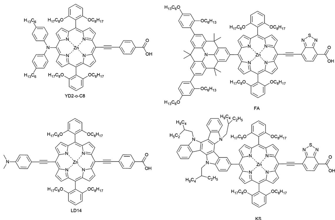
Fig. 15 Chemical structures of porphyrin-based sensitizers for ssDSCs.
