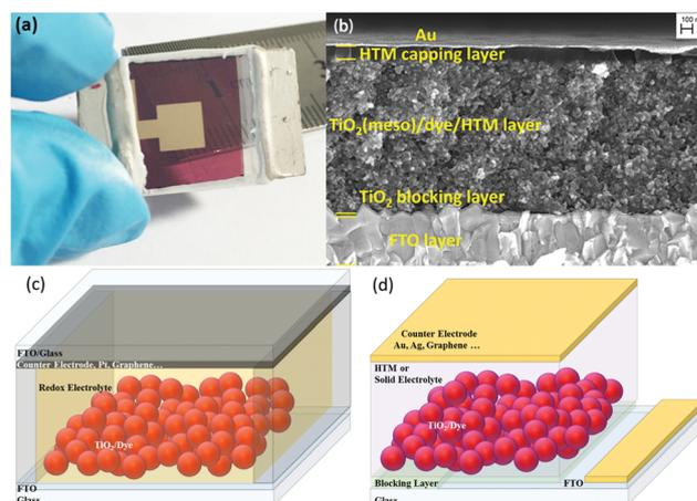
**Fig. 1** (a) A fully assembled ssDSC with a Au counter electrode. (b) Cross-sectional electron microscopy image of a ssDSC. Adapted with permission from ref. 78. Copyright 2016 American Chemical Society. (c) Schematic sketch of solar cell architectures for the assembly of liquid-junction DSCs and (d) ssDSCs.
