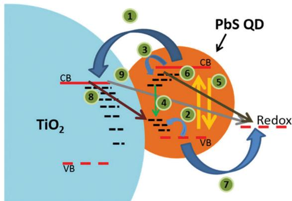
Fig. 19 Schematic illustration of photoinduced charge-transfer processes following absorption of quanta of light by PbS QDs on TiO<sub>2</sub>. Reprinted from ref. 190 with permission from the American Chemical Society.
