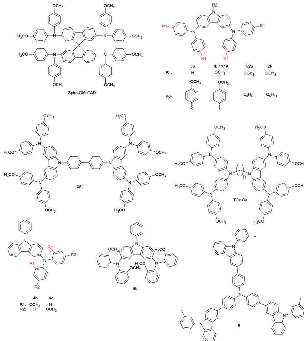
Fig. 22 Spiro-OMeTAD and novel carbazole-based hole transport materials.
