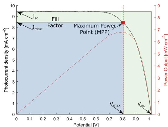
Fig. 4 Characteristic *I*-*V* scan of a ssDSC.
