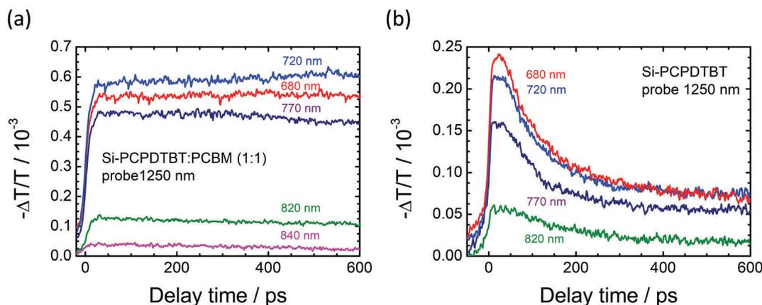
**Fig. 3** Transient absorption spectra of Si-PCPDTBT blended with PCBM (1:1 ratio) upon pumping at different wavelengths (a). The probe wavelength was fixed to 1250 nm and is sensitive to both the exciton and polaron population. The long lasting signal indicates the formation of polarons. The decay curves for the neat polymer in (b) are marked by a fast initial decay due to exciton recombination and exhibit a finite signal for long delays due to polaron absorption.
