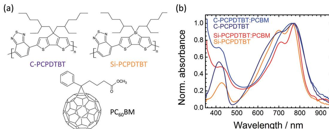
Fig. 2 Molecular structure of C-/Si-PCPDTBT and the electron acceptor PC<sub>60</sub>BM (a). The substitution of the bridging atom of the side-chains has a profound impact on the polymer morphology. The normalised absorbance spectra of cast thin films of neat polymers and 1 : 1 blends with PC<sub>60</sub>BM exhibit two absorption bands for both polymers (b). Vibrational subpeaks form for the Si variant due to chain aggregation.
