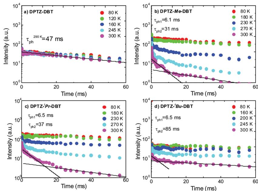
Fig. 8 Time resolved phosphorescence decays in zeonex obtained as a function of temperature for (a) **DPTZ-DBT**, (b) **DPTZ-Me-DBT**, (c) **DPTZ-<sup>1</sup>Pr-DBT** and (d) **DPTZ-<sup>4</sup>Bu-DBT**.
