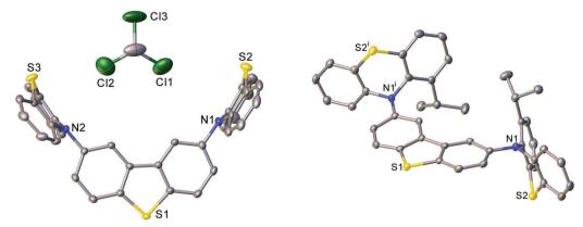
Fig. 2 X-ray molecular structures of DPTZ-DBT·CDCl<sub>3</sub> (left) and DPTZ-iPr-DBT (right) showing equatorial and axial PTZ groups, respectively. Thermal ellipsoids are drawn at the 50% probability level; H atoms are omitted; primed atoms are generated by the twofold axis.
