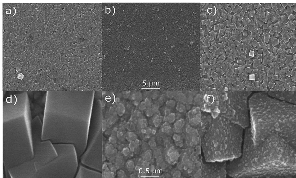
**Fig. 2** SEM analysis at different zoom levels, showing the FeCr (a and d), FeFe (b and e) and the bilayer films (c and f). The FeFe film can be seen in image (f) as the smaller crystals on the surface of the larger FeCr crystals. The smaller structures visible below the FeCr crystals in (d) is the conductive FTO layer on the glass substrates.  $5 \mu\text{m}$  scale bar refers to images a–c while the  $0.5 \mu\text{m}$  scale bar refers to images d–f.
