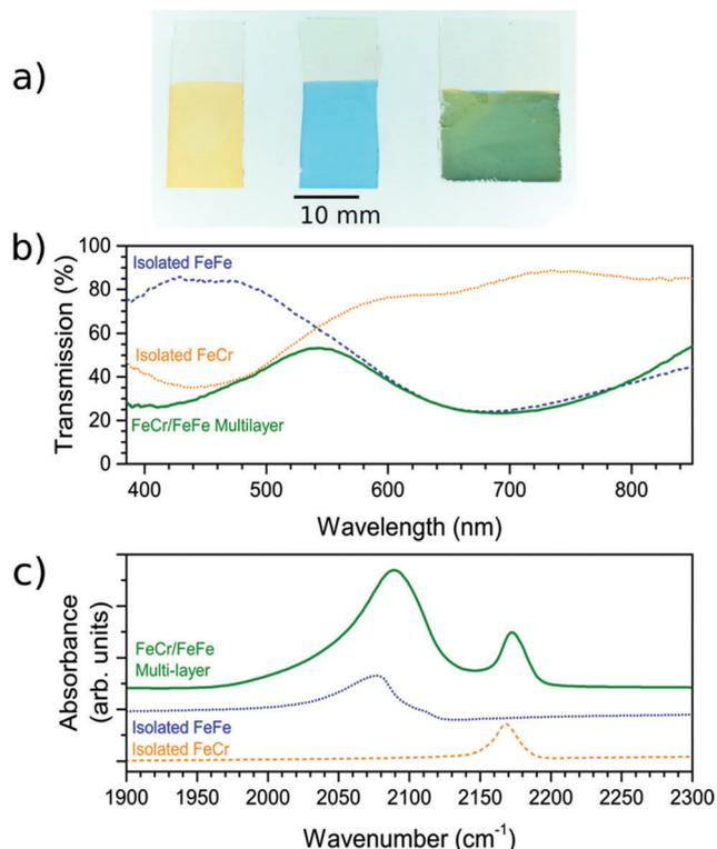
**Fig. 1** Visible transmission and IR spectra of the individual and the bilayer films. (a) Photos of the FeCr (orange, left), FeFe (blue, middle) and FeCr–FeFe bilayer structure (green, right). (b) Transmission spectra for the FeCr, FeFe films and the bilayer material. (c) The IR spectra showing the CN<sup>−</sup> stretching frequencies of the FeCr and FeFe films, and those present in the bilayer. The IR spectra have been vertically offset for clarity.
