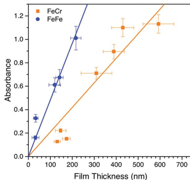
**Fig. 4** The dependence of the optical density on the thickness of the film for the FeFe and FeCr Prussian blues. The error bars come from the AFM/UV-Vis analysis performed on the deposited samples, many cross sections/spots of the film were taken to reliably estimate these values. Note the error in absorption data increases with larger film thickness due to larger amount of scattered light as the crystals become larger.
