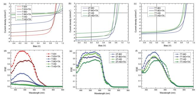
Fig. 4 (a-c) J-V-characteristics of optimized bulk heterojunction solar cells of PDCB polymers containing (a) thiophene, (b), bithiophene, and (c) thienothiophene with PC<sub>71</sub>BM. (d-f) Corresponding EQE spectra of the same devices. TA is thermal annealing for 10 min at 120 °C
