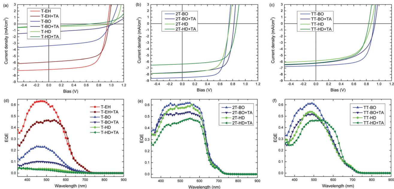
Fig. 4 (a–c)  $J$ - $V$ -characteristics of optimized bulk heterojunction solar cells of PDCB polymers containing (a) thiophene, (b) bithiophene, and (c) thienothiophene with PC<sub>71</sub>BM. (d–f) Corresponding EQE spectra of the same devices. TA is thermal annealing for 10 min at 120 °C.
