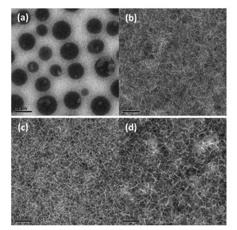
Fig. 5 Bright-field TEM micrographs of optimized, pristine active layer blends with PC71BM for (a) PDCB-T-HD; (b) PDCB-2T-BO; (c) PDCB-2T-HD. (d) A thermally annealed blend of PDCB-2T-HD:PC71BM. In each case, the mixing ratio was 1:1.5 (polymer/fullerene) by weight.
