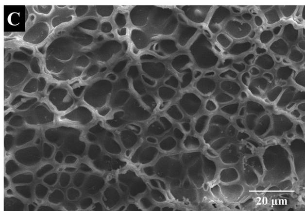
Fig. 3 SEM images of lyophilized hydrogels, prepared with TCS2-5 and different concentrations of ChA: (A) 0.24TCS2-5; (B) 0.49TCS2-5; and (C) 0.73TCS2-5. Magnification  $\times 1000$ . At least twenty pores per each SEM image were taken into account for the calculation of the hydrogel average pore size.
