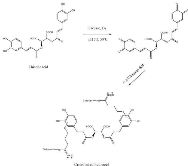
**Scheme 1** Schematic representation of the laccase-assisted hydrogel formation between TCS and ChA. The one-step hydrogel synthesis can be subdivided into two consequent reactions. In the first reaction, phenolic groups of ChA are oxidised by laccase, yielding quinone derivatives. In the second reaction, two molecules of TCS are chemically crosslinked through Michael-addition reaction of nucleophilic thiol groups and quinone moieties.
