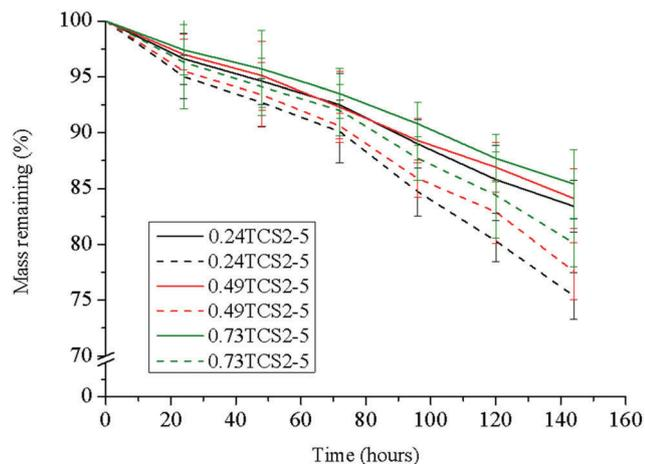
Fig. 6 Stability of hydrogels in PBS alone (continuous line) and in the presence of lysozyme (dashed line). The hydrogels were prepared with TCS2-5 and various ChA concentrations. The results are reported as mean values  $\pm$  SD ( $n = 5$ ) and their statistical significance was calculated using one-way ANOVA ( $p < 0.05$ ).
