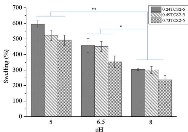
Fig. 4 Swelling behavior of hydrogels prepared from TCS2-5 and varying the concentration of ChA at different physiological pHs. The results are reported as mean values  $\pm$  SD ( $n = 5$ ) and their statistical significance was calculated using one-way ANOVA ( $p < 0.05$ ).
