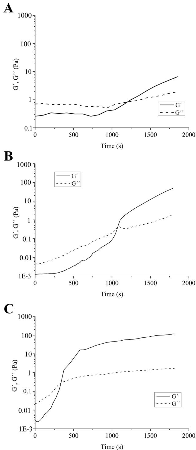
**Fig. 1** Time sweep rheological characterization of the hydrogels. Evolution of the storage ( $G'$ ) and loss ( $G''$ ) moduli vs. time at 50 °C of hydrogels, prepared with the highest degree of thiolation and the same concentration of ChA in the presence of laccase (2.7 U mL<sup>-1</sup>), (A) 0.73TCS1-10, (B) 0.73TCS1-5 and (C) 0.73TCS2-5.
